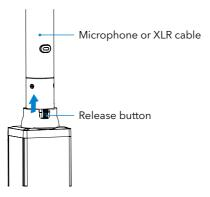
**2** Disconnect a microphone or XLR cable. Press the release button and pull the microphone or XLR cable out carefully in the direction of arrow.
